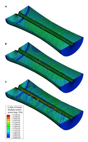
Figure 4. Distribution of the maximum principal strain on the finite element (FE) model; a cross-section showing the effect of the load transfer via the trabeculae
