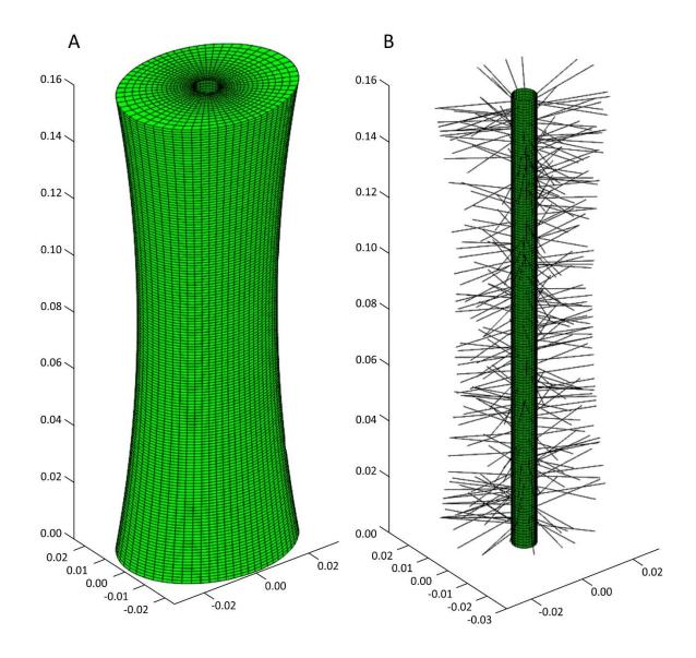
**Figure S3**. Computational mesh: (A) external wall and top lid; (B) detail of the internal structure: the internal neural tube is connected to the external vertebral wall by radial trabeculae, randomly arranged on the total bone marrow space and producing a "spoke-like" structure. This schematic based on XCT scans of specimen in Figure 1 and seen in Figure 2.
